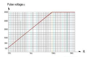
Pulse load rating in accordance with IEC 60115-1,4.27;  $1.2\mu s/50\mu s$ ; 5 pulses loaded, for permissible resistance change  $<\pm(0.5\%+0.05\Omega)$
