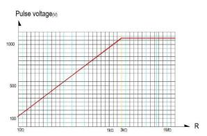
Pulse load rating in accordance with IEC 60115-1,4.27;  $10\mu s/700\mu s$ ; 10 pulses loaded, for permissible resistance change  $<\pm$ (0.5%+0.05 $\Omega$ )
